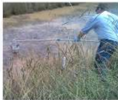
Sampling of six bottles at one time from the centre of the channel without entering into the channel
