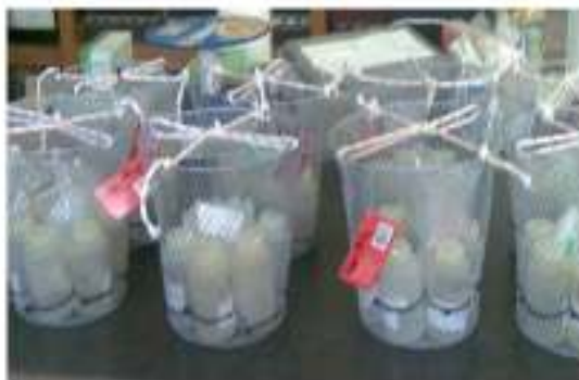
Six nalgene bottles tied together to a basket using cable ties
